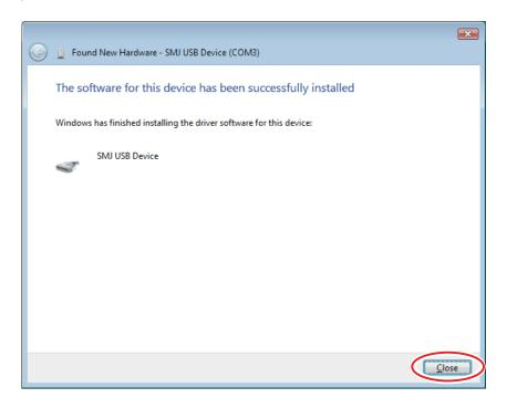
9. From the property of My Computer, select [Device Manager] and confirm that **SMJ USB Device** (Com\*) appears under Ports (Com & LPT). If it does, installation has completed successfully.
