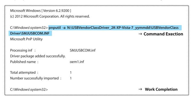
4. Connect the Star Printer or Visual Card-Reader/Writer to the computer with a USB cable, and turn on the Star Printer or Visual Card-Reader/Writer with the power switch. The computer detects the new hardware and installs the USB Vendor Class Driver with Plug and Play. Close the command prompt .
