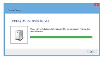
5. From the [All apps]-[Control Panel], select [ Device Manager ] and confirm that **SMJ USB Device (Com\*)** appears under **Ports (Com & LPT)** . If it does, installation has completed successfully.
